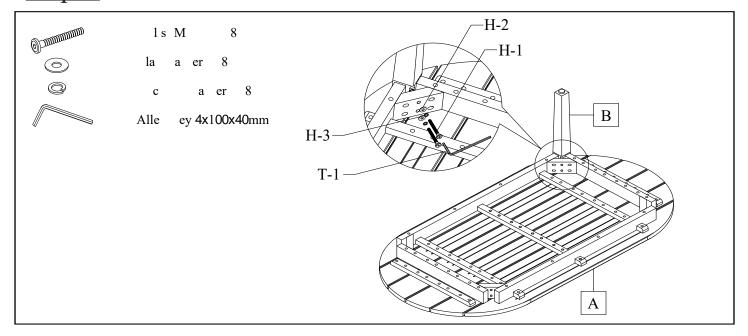
Using a second person to assist you, lay Table Top (A) upside down onto a padded, non-marring surface. Secure one Leg (B) to the Table Top (A) with the Bolts (H-1), Flat Washers (H-2) and Locking Washers (H-3) using the provided Allen Key (T-1), stacking the hardware in the order as shown. Fully tighten all hardware but DO NOT OVER TIGHTEN. Repeat the same process for the remaining Legs (B) at each corner of the apron.
